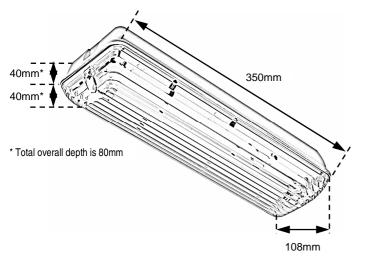
Cut-Out Dimensions:Length 330mm x Width 90mmViewing Distance:18 Metres (when supplied with SAL1 legend kit)
